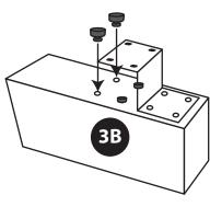
When mounting the newspaper holder on a single post, simply align the elongated holes on the newspaper bracket with the holes with the top of the post figure **4A**. Align the holes in the mounting bracket with the Mail Boss or Fast track on top. Then, secure the mailboss to the newspaper holder bracket and the post using a 13 mm socket or wrench.
