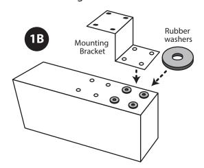
Center the 4 rubber washers over the 4 holes in the top which are closest to the **REAR** of the newspaper holder. Line up the 4 circular holes in the bracket with the holes on the rubber washers. Make sure the elongated holes in the bracket are centered over the newspaper holder as shown in figure **1B**.
