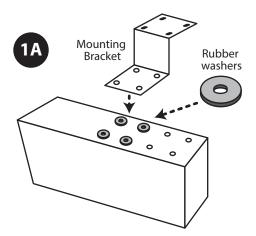
Center the four rubber washers over the 4 holes in the top of the holder that are the closest to the front opening. Line up the circular holes in the bracket with the holes on the rubber washers as shown in figure **1A**.
