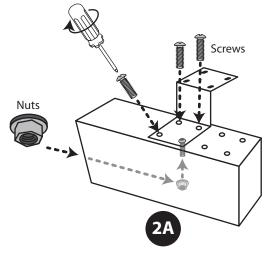
Insert the four stainless steel machine screws through the top and into the newspaper holder as displayed in figure **2B**. While pressing each screw down with your thumb, finger tighten the stainless steel nuts, flange first, on the inside of the newspaper holder. Using a #2 Phillips screw driver, tighten each of these screws.
