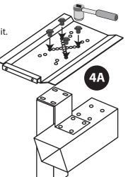
Use these instructions to mount a newspaper holder to our Mail Boss spreader plates (with the exception of the center of a triple spreader). Mount the spreader plate to the post as described in the spreader plate installation instructions. Align the elongated holes on the newspaper holder bracket with the top of the post.
