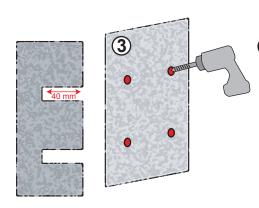
Using the 4 mm drill bit provided, create four pilot holes at least 10 mm deeper than screws provided, or about 40 mm deep. If the material is unusually hard you may need to use a rotary impact drill rather than a standard drill to make the holes. Call a handy man if needed. Put a small amount of caulk or silicone into each hole.
