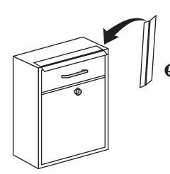
**OPTIONAL:** If you're installing this box in a location without overhead weather protection, you may wish to install the rain guard weather shield on the top of your box for added moisture protection. Simply remove the adhesive backing from the rain guard and install upon the front of the upper ledge of the box, with the lip overhanging the upper door.
